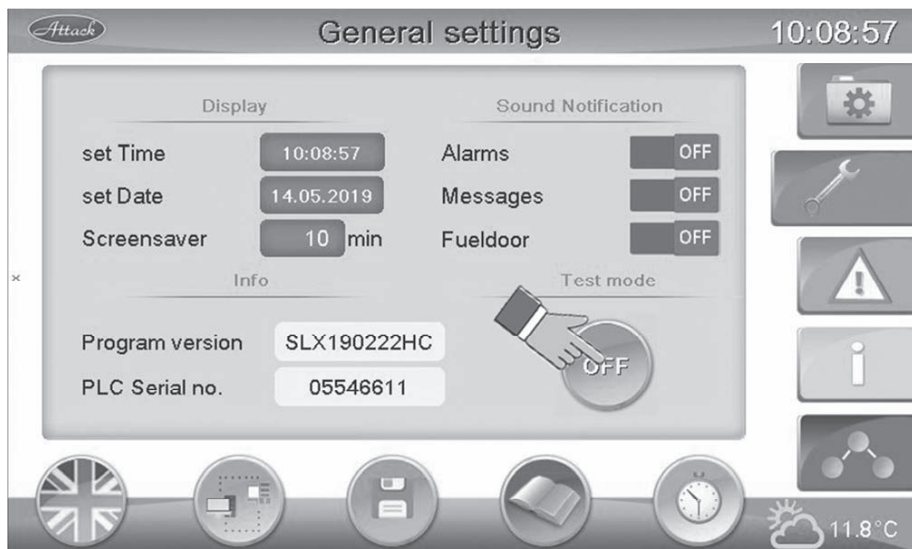
Pic. 24 Finishing of the boiler's test mode
