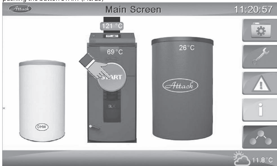
Pic. 25 Boiler start on
